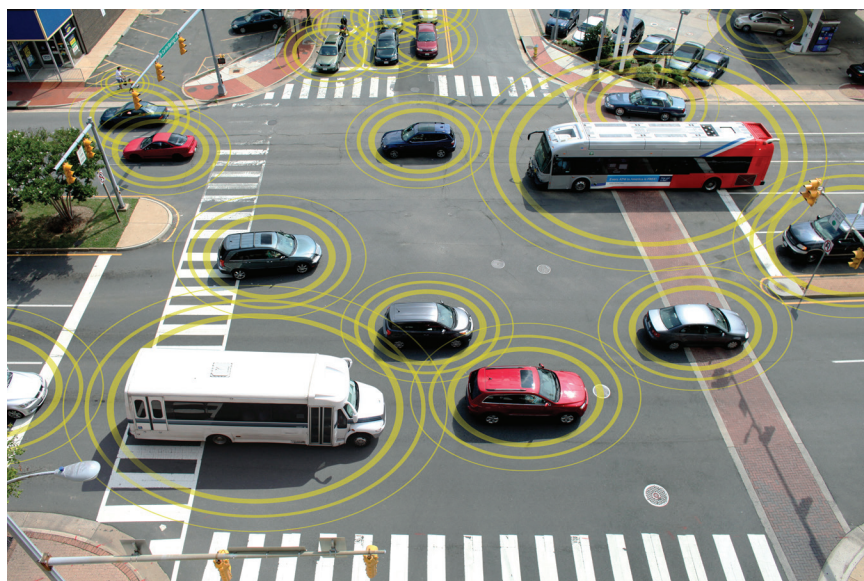
Figure 4.5. Vehicle-to-vehicle and vehicle-to-infrastructure technology (National Highway Traffic Safety Administration)
